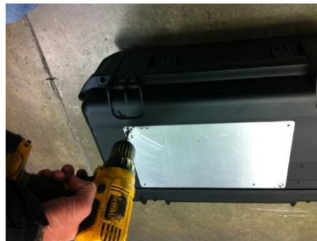
Insert a screw into each hole as you drill them to hold alignment
