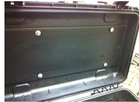
Push sealing washers onto the screws, note that they will be very tight because they have a rubber backing which allows them to seal the case.
